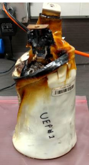
Melted Down Cell Following Heat Exposure Test, No Fire!
