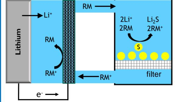
reduce solid, energy-storing sulfur particles kept in the catholyte reservoir tank. Catholyte is flowed into an electrochemical cell where electrons are extracted from mediators at a porous carbon electrode.
