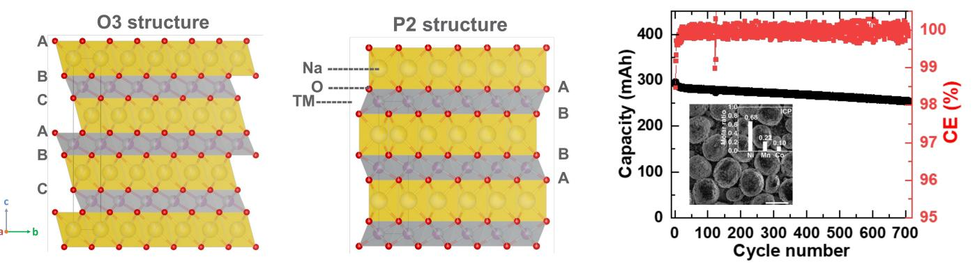
The O3 NaNi<sub>0.6</sub>Mn<sub>0.2</sub>Co<sub>0.2</sub>O<sub>2</sub>-hard carbon pouch cells (~300 mAh) delivered ~88% retention over 700 cycles. The viability of sodium-ion battery was demonstrated.
