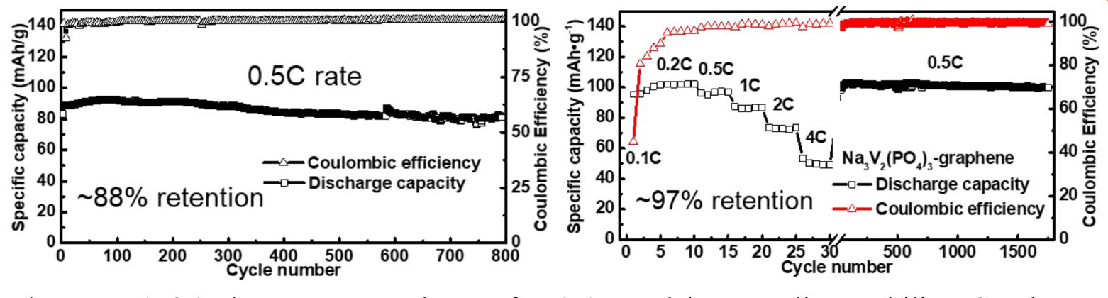
Na<sub>3</sub>V<sub>2</sub>(PO<sub>4</sub>)<sub>3</sub> has average voltage of ~ 3.4V and long cycling stability. Graphene coated Na<sub>3</sub>V<sub>2</sub>(PO<sub>4</sub>)<sub>3</sub> demonstrated improved rate performance and cycling stability with ~97% capacity retention over 1500 cycles.
