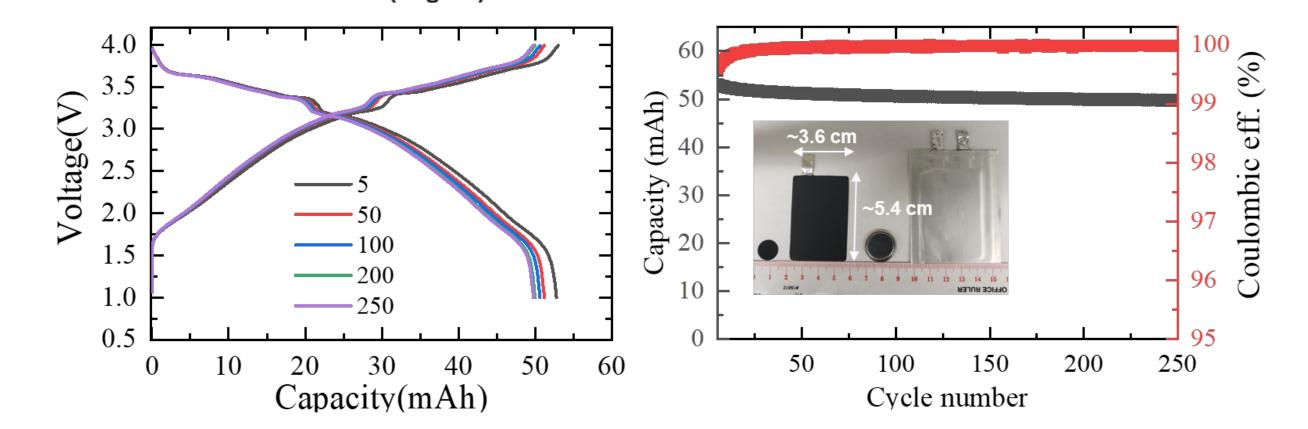
The single layer pouch cell of P2/O3 Na<sub>0.85</sub>Mn<sub>0.5</sub>Ni<sub>0.4</sub>Fe<sub>0.1</sub>O<sub>2</sub>-hard carbon (~50 mAh) has demonstrated ~94% retention over 250 cycles.
