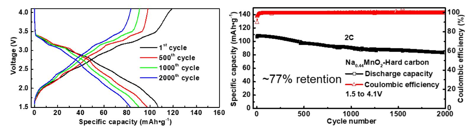
The full cell demonstrated ~77% retention over long term cycling (2000 cycles).
