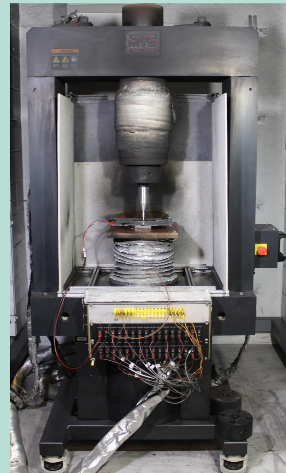
Hydraulic equipment with 6mm indenter
