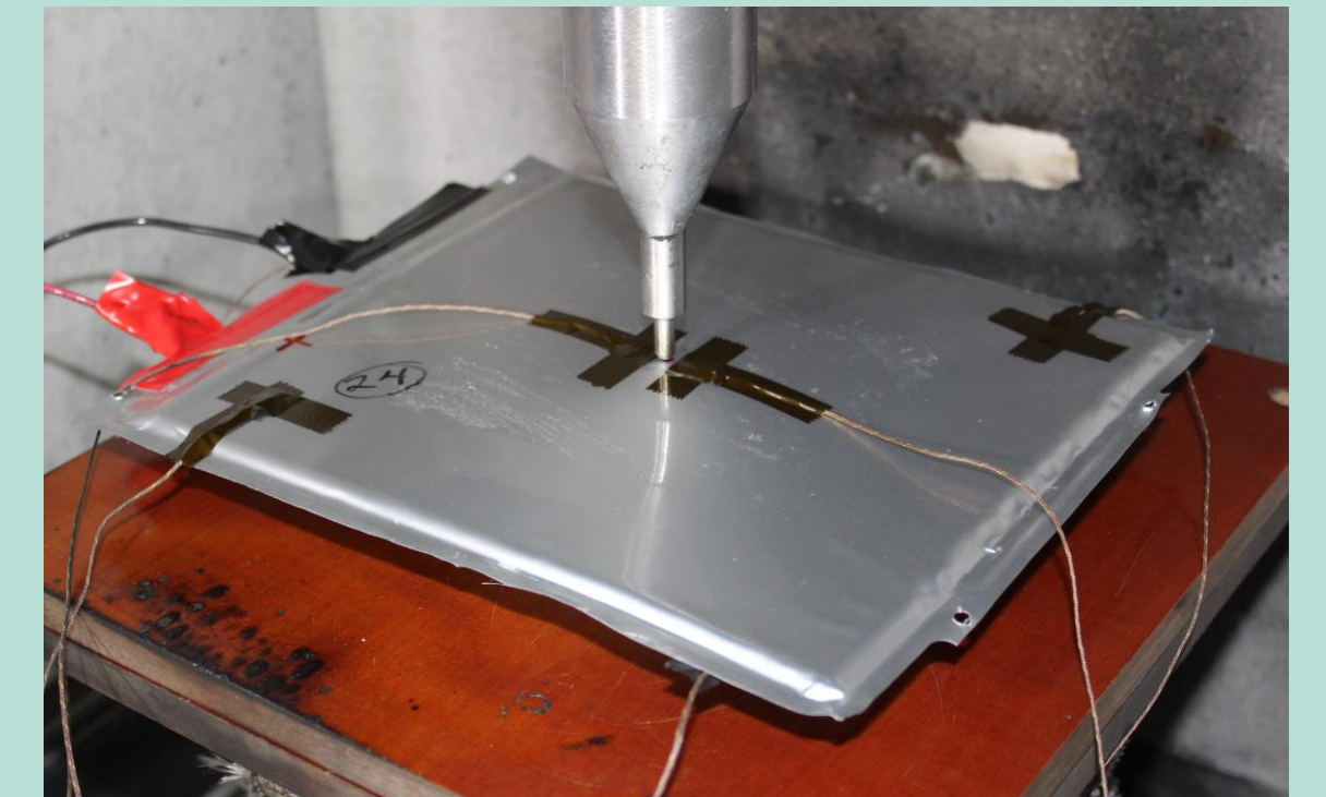
Single cell prepped for testing with voltage sense leads and thermocouples
