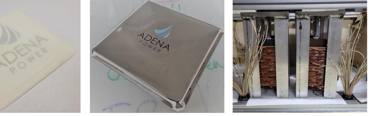
Building block module ~ 3.75 kWh
