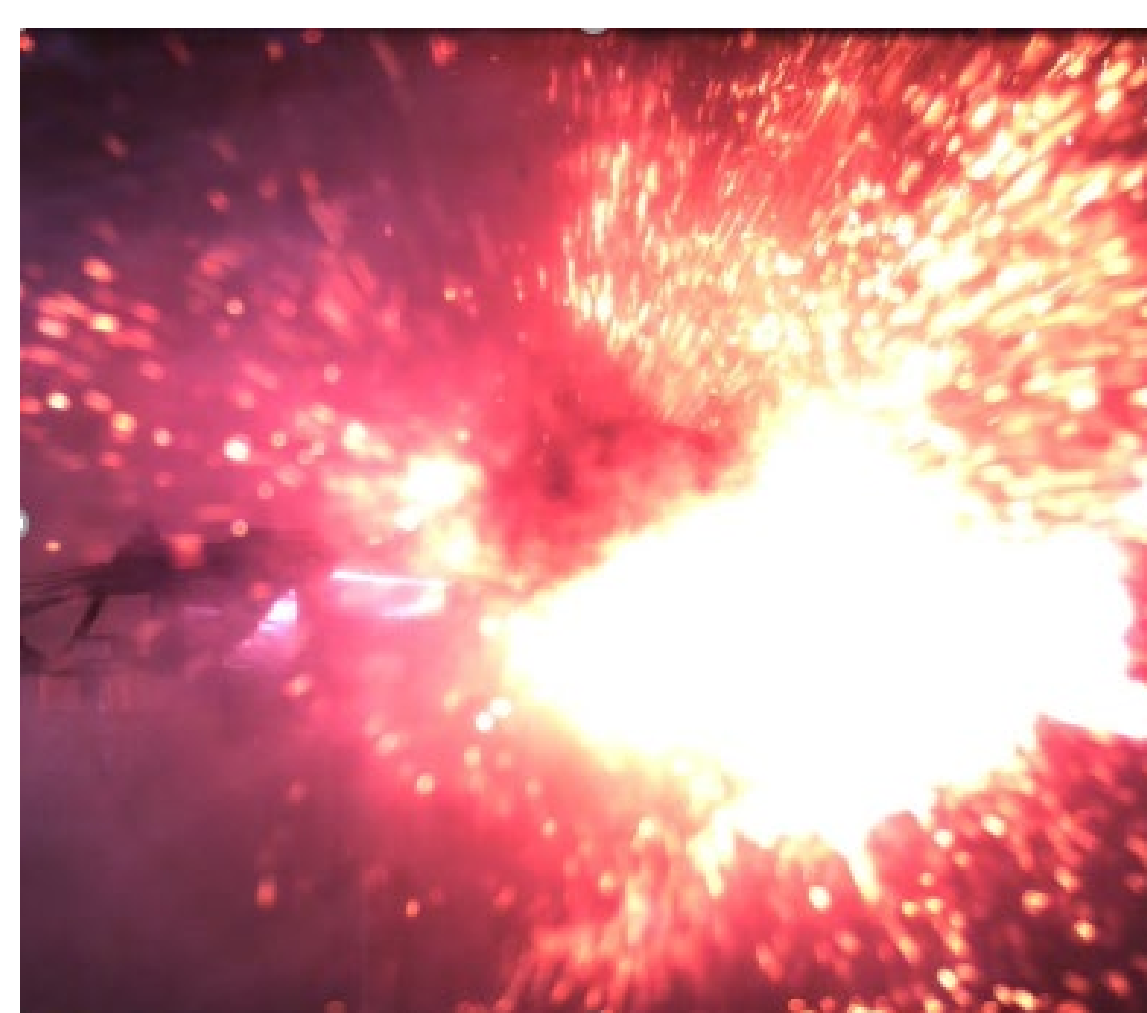
Figure 1: Failing 18650 format cell
