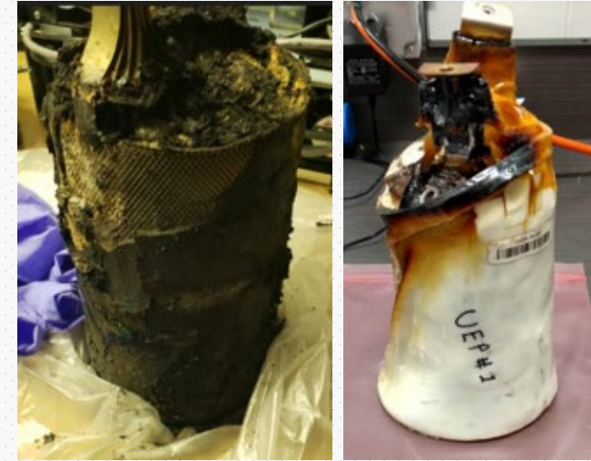
UEP Zn-MnO 2 batteries after 9540A testing (above) and temperature data captured during the test (below).
