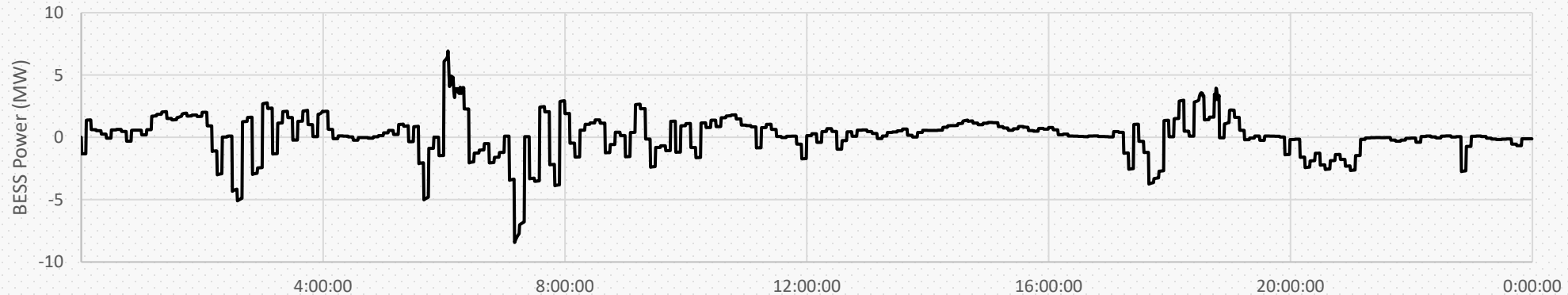
Real 10 MW BESS power data in a typical day
