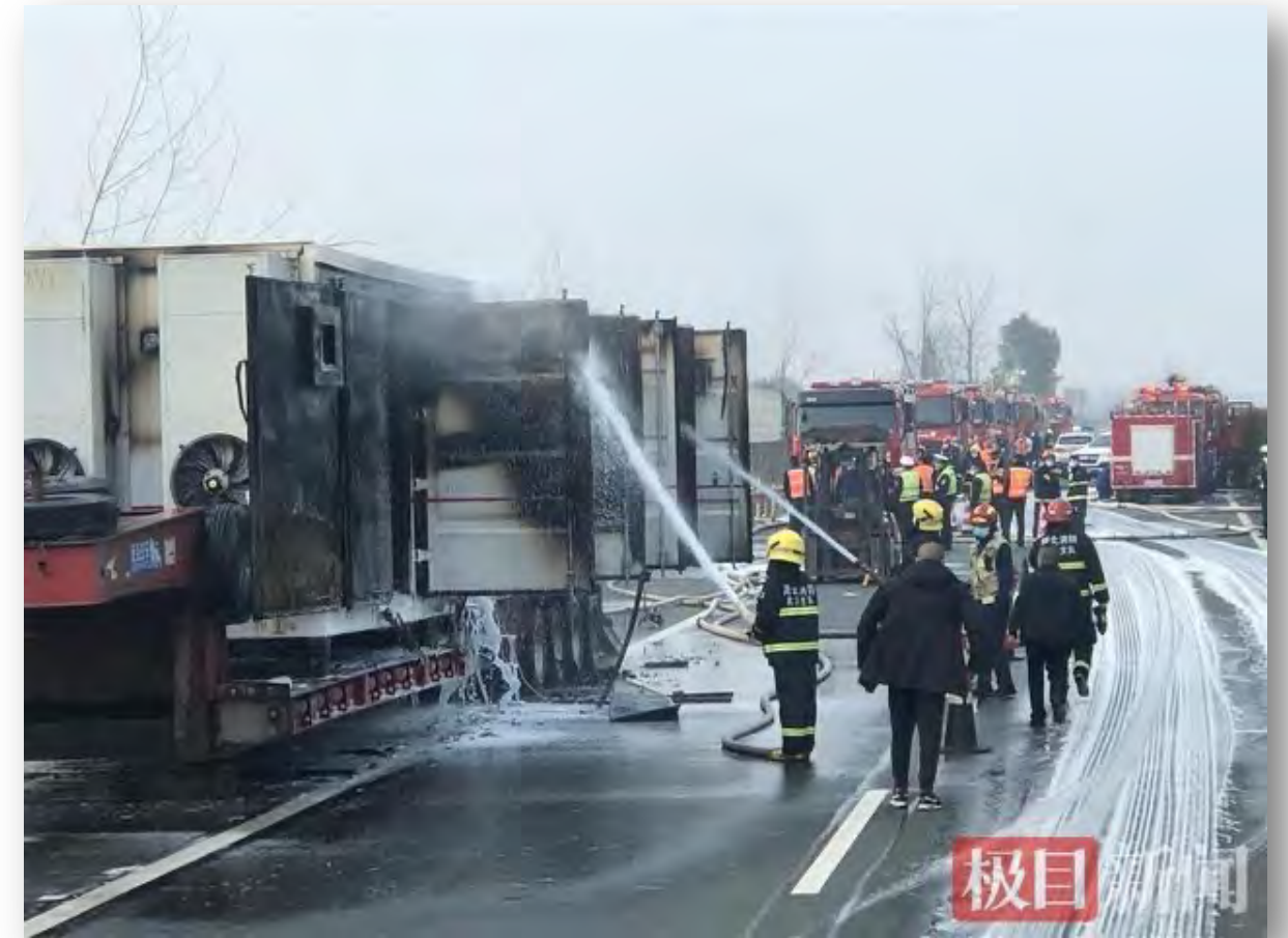
New ESS in transport w/LFP cells
