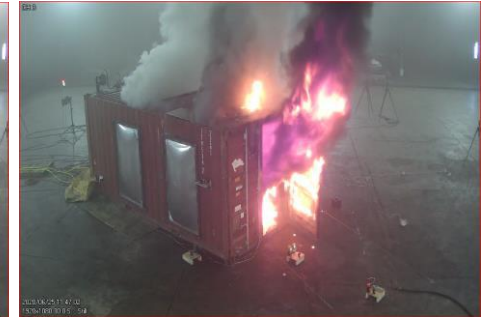
Flashover and flaming from open door [TR + 02:09:48]
