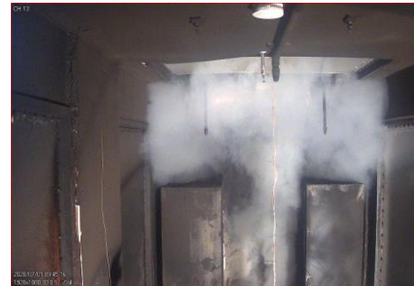
Smoke accumulation and first response of LEL at the ceiling [TR + 00:00:29]
