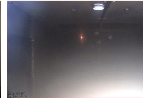
Smoke stratification before ignition [TR + 00:26:51]
