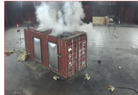
Continued thermal runaway propagation [TR + 00:46:26]
