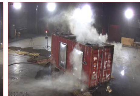
Thermal runaway propagation after end of water flow [TR + 01:13:05]
