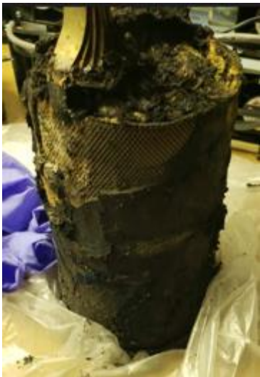
UEP Zn-MnO 2 batteries after 9540A testing (above) and temperature data captured during the test (below).
