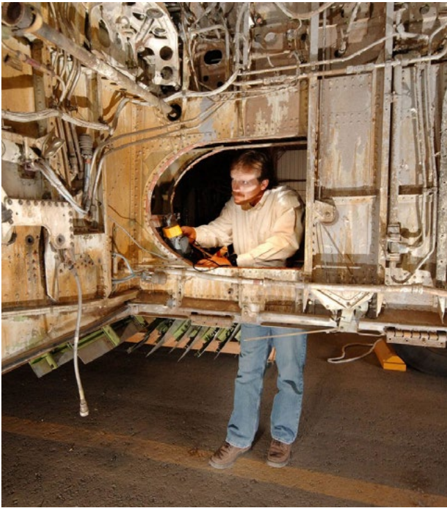
AIRCRAFT SAFETY — Sandian Kevin Howard inspects electrical wiring in the wheel well of a retired Boeing 727 in this 2006 photograph.
