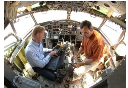
WIRING DIAGNOSTIC — Sandians Larry Schneider, left, and Mike Dinallo prepare to employ the Pulse Arrested Spark Discharge diagnostic in 2006 on a wiring bundle in the cockpit of a retired Boeing 737. Photo by Randy Montoya
