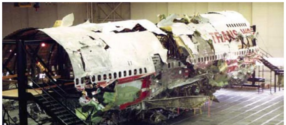
TWA 800 — A photograph from the National Transportation Safety Board’s final report shows wreckage from the crash reconstructed in a hangar in New York.
