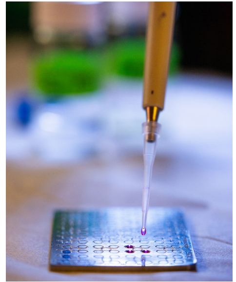
SAMPLE — Chemist Samantha Kruse preps a sample for the Matrix-Assisted Laser Desorption Ionization analysis. Photo by Craig Fritz
