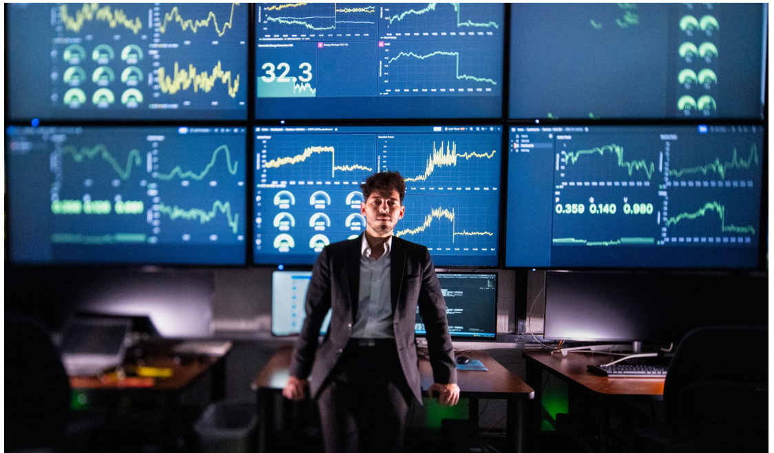
DASHBOARD VIEW — In Sandia’s Distributed Energy Technologies Laboratory, engineer Rachid Darbali-Zamora reviews the DERMS control dashboard used to coordinate grid-connected devices such as inverters, batteries and solar resources. The AI-enabled controls are being tested to improve voltage regulation and power quality for sensitive loads.
