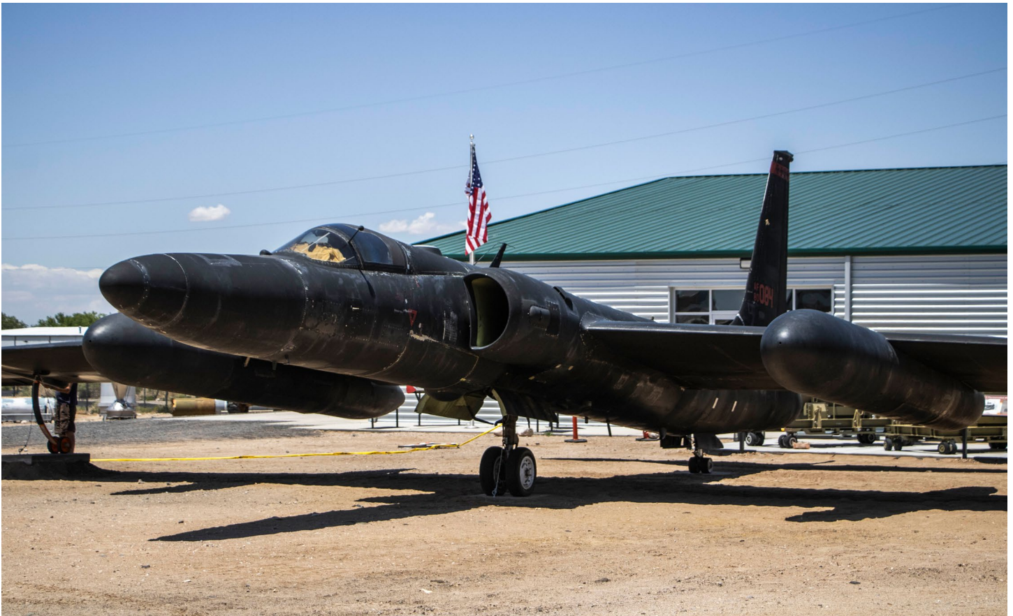
FULLY ASSEMBLED — The Lockheed U-2 Dragon Lady is on display in Heritage Park at the National Museum of Nuclear Science & History in Albuquerque after days of rebuilding by Worldwide Aircraft Recovery, a team based in Bellevue, Nebraska, that provides such services as plane disassembly and reassembly. The Dragon Lady is a single-engine, single-seat aircraft that has been used for intelligence-gathering from altitudes above 70,000 feet since the 1950s.
