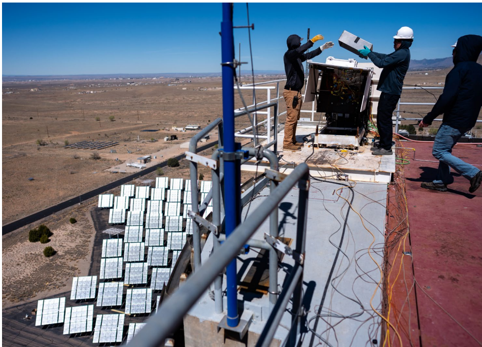
SET UP — Sandia engineers Aaron Overacker, left, Todd Arterburn, and Lockheed Martin engineer Derek Shannon, right, get ready to test heat shield material samples at the National Solar Thermal Test Facility for NASA's Dragonfly mission to Titan.
