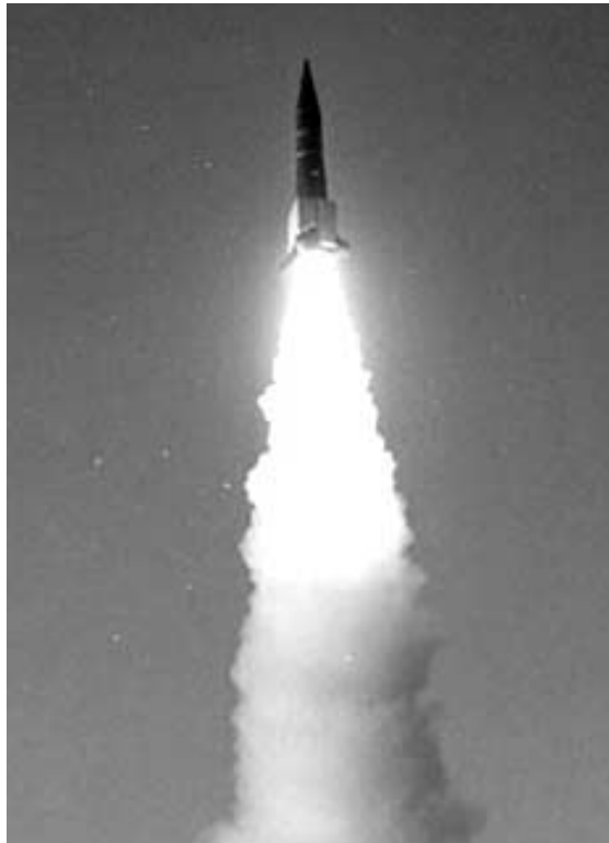
TARGET VEHICLE (based on a modified Minuteman I second stage rocket motor) lifts off from the Kauai Test Facility Jan. 25. (Photo by Diana Helgesen, 15419)
