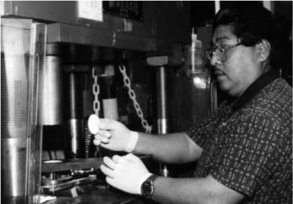
PELLET COMPRESSING — Joe Garcia (2522) inspects a compressed powder pellet similar to those used in the MC3323A batteries that members of the Power Sources Technology Group in Center 2500 produced and delivered in record time to support DOE flight tests. For their efforts they were recently awarded the DOE Weapons Recognition of Excellence Award and were commended in a December 2000 DOE quality Assurance Survey Report. (Photos by Chris Burroughs)
