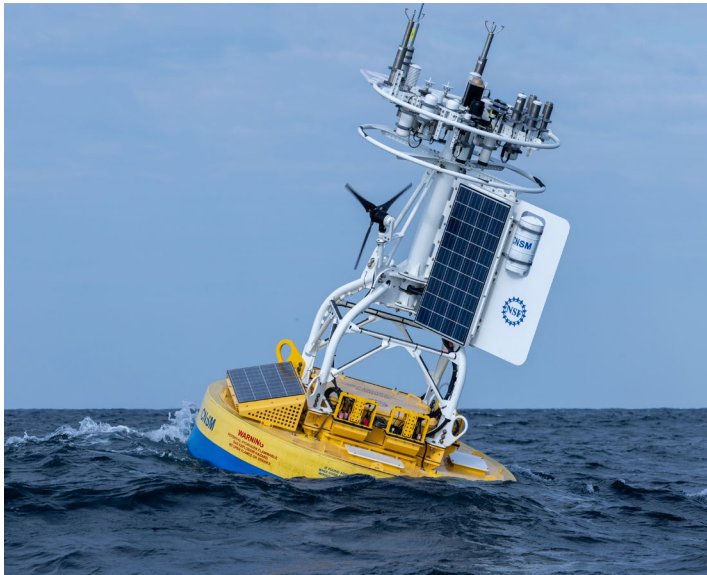
WAVE RIDER — The Ocean Observatories Initiative Pioneer Array coastal surface moorings buoy. Photo by Taylor Mankle and Joshua Bauer, National Laboratory of the Rockies
