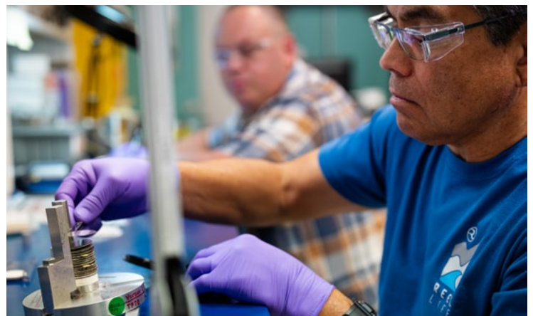
QUALITY CHECKS — A Sandia technologist works on a thin film thermal battery as his colleague performs quality assurance checks for the Power Sources Capabilities team. Photo by Craig Fritz
