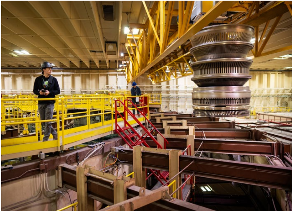
MIGHTY MITL — Sandia technologists Alex Nash, left, and Jacob Werner transport the Saturn Accelerator’s magnetically insulated transmission lines, from the center section for cleaning after a shot.
