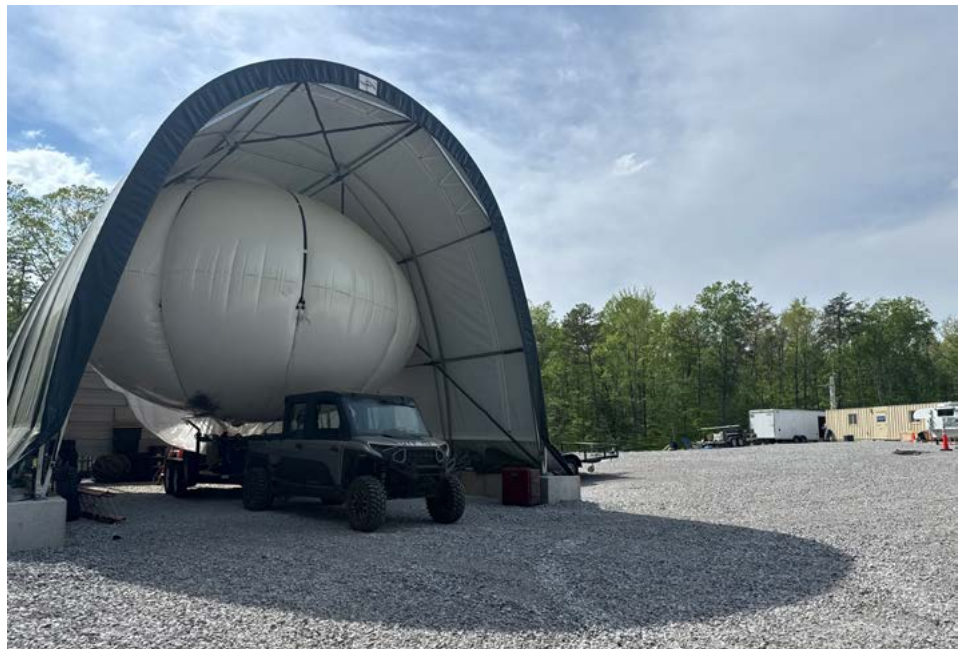
BALLOON SETUP — The typical footprint of a tethered balloon field campaign consists of the balloon and launch vehicle, a temporary hangar and three to five containers or trailers. Photo by Antigravity Films
