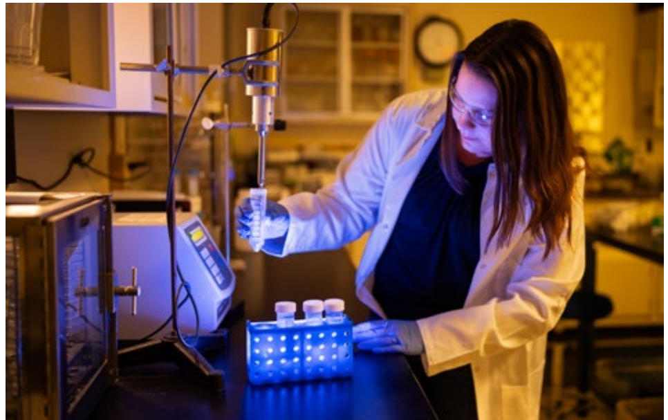
IN THE MIX — Jessica Rimsza uses a sonication probe to thoroughly mix powder in a solvent to make porous liquid for further testing. Photo by Craig Fritz
