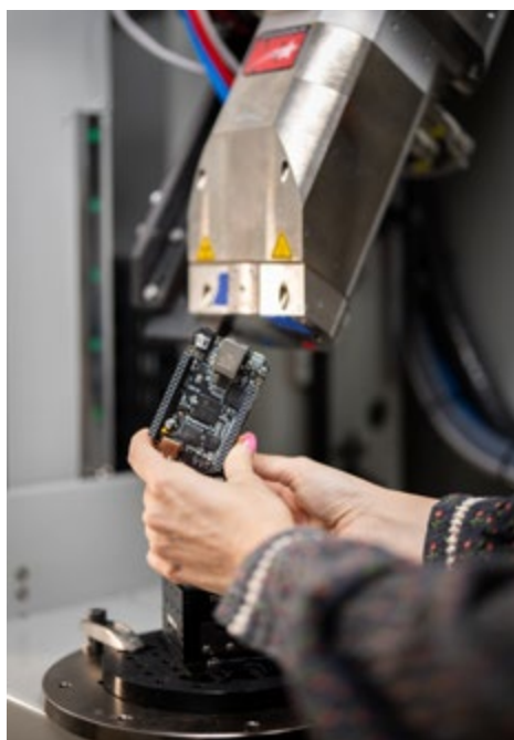
MULTI-METAL POWER — Noelle Collins sets up for an X-ray CT scan of a circuit board as part of the Non-Destructive Evaluation group at Sandia. Photo by Craig Fritz
