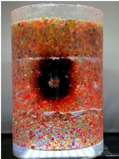
BLEEDING REVEAL — A container protected with Sandia's "Bleeding Materials and Enclosures" product indicates a tamper attempt. In this image, silicone is used to encapsulate the air-sensitive beads.
