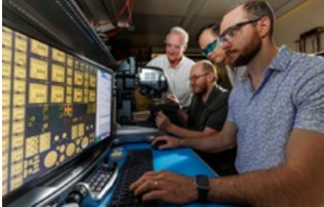
CLOSER LOOK — Examination of record-setting hafnated GaN MOSFETs under an optical microscope. Photo by Craig Fritz
