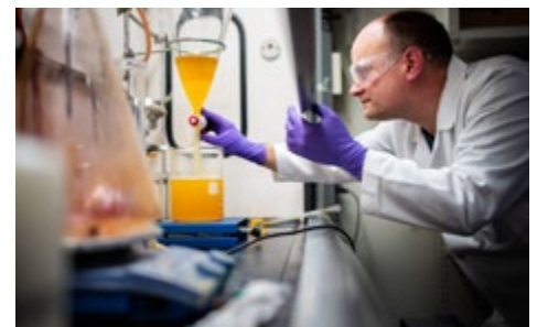
CHEMISTRY AT WORK — Sandia chemist Chad Staiger uses a separatory funnel to remove byproduct from the synthesis of a molecule.
