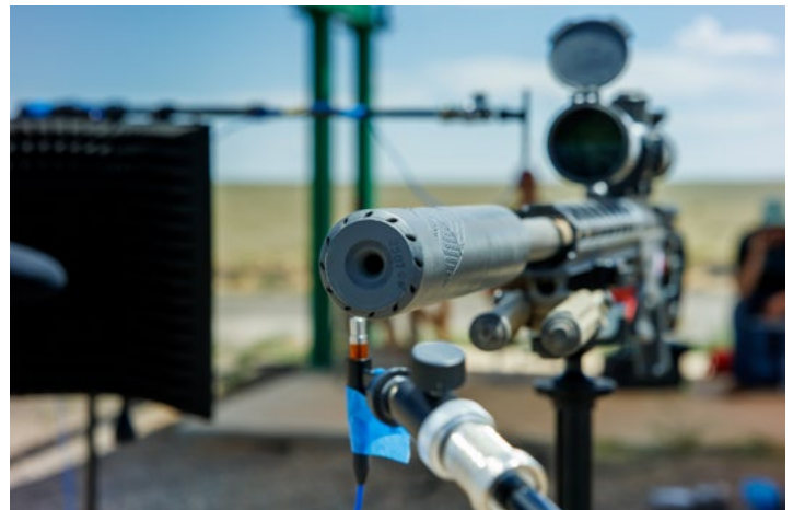
SURROUND SOUND — Sandia engineers placed multiple microphones around a Ridgeline Manufacturing suppressor during testing to record the sound at different points, then analyzed the data to determine impact on the human ear. Photo by Bret Latter
