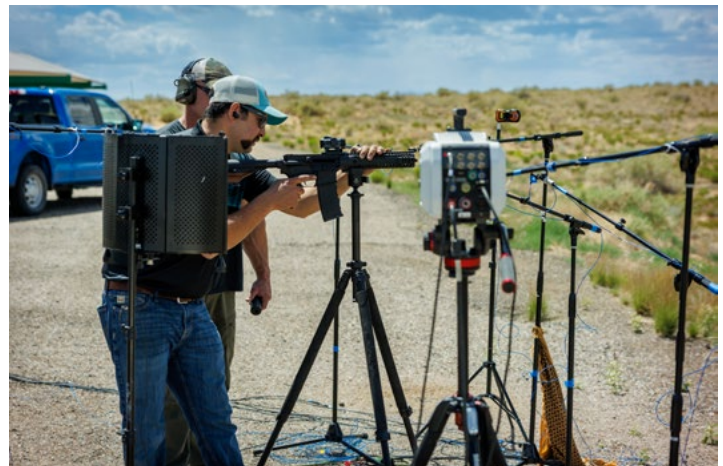
PRECISION SOUND — Matias Roybal and a fellow member of the Ridgeline team conduct high-fidelity acoustic tests on their suppressors with the help of Sandia acoustics and vibration engineers. Photo by Bret Latter
