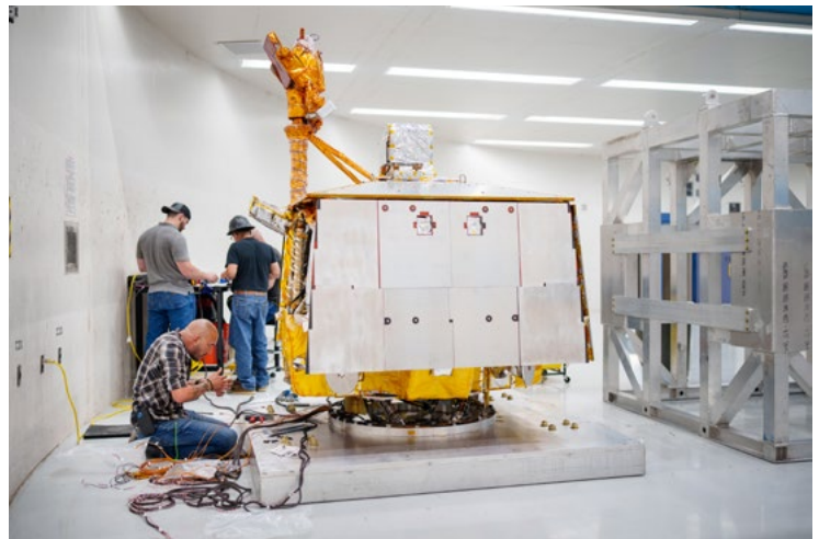
WIRING THE MISSION — Operations engineer Orlando Abeyta works on wiring prior to placing a cage around and attaching VIPER to the arm of the Superfuge at Sandia. Photo by Craig Fritz
