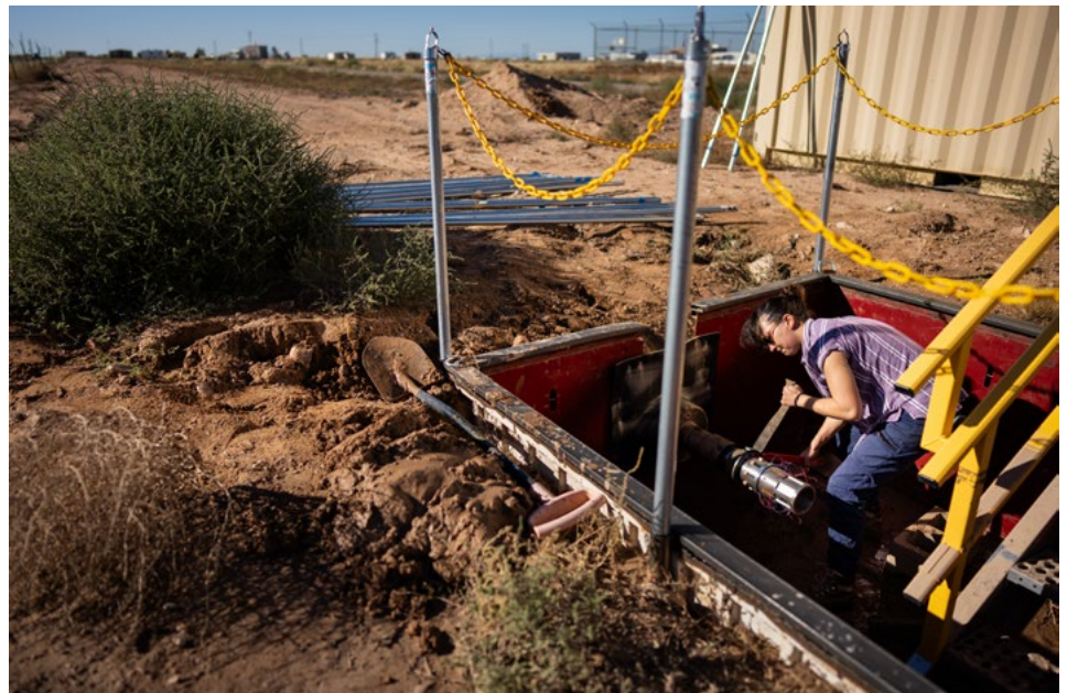
PROTOTYPE PREPARATION — Melanie Schneider prepares the testbed for the evaluation and optimization of an innovative prototype that leverages the casing string as an acoustic waveguide to enable wireless power and communication for downhole sensors. Photo by Craig Fritz
