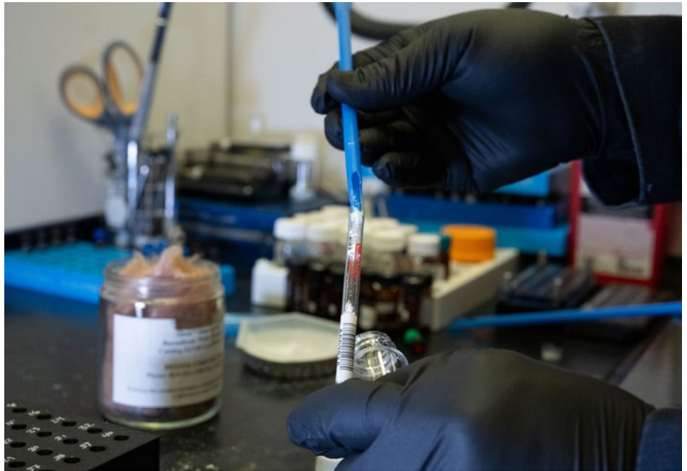
CAPTURING COMPOUNDS —Chemist Jason Sammon packs a glass sorbent tube with the metal-organic framework powder, which forms the preconcentrator to capture volatile organic compounds.
