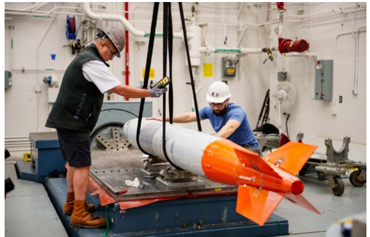
EARLY DELIVERY — A B61-13 vibration fly around unit is prepared for testing on a shaker table at Sandia. Assembly of the first production unit was completed at the Pantex Plant in May, about a year ahead of schedule.
