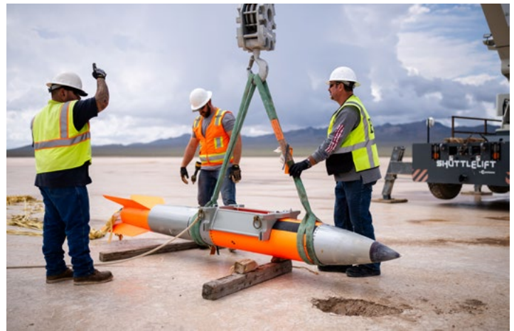
TEST TIME — Navarro Engineering and Research contractors recover a mock B61-4 for analysis, following a drop by an F-15 in 2022.
