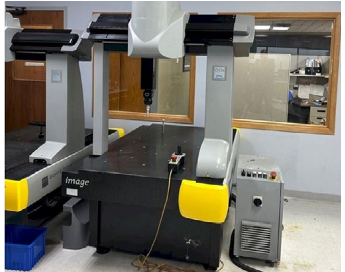
MEASURE TWICE — The coordinate measuring machine donated by Sandia can check parts that measure tens of thousandths of an inch.
