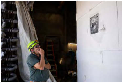
HOT STUFF — In a photo from 2022, a lead technologist at Sandia’s National Solar Thermal Test Facility assesses damage to some aerospace heat-shield materials after on-sun testing. Photo by Craig Fritz
