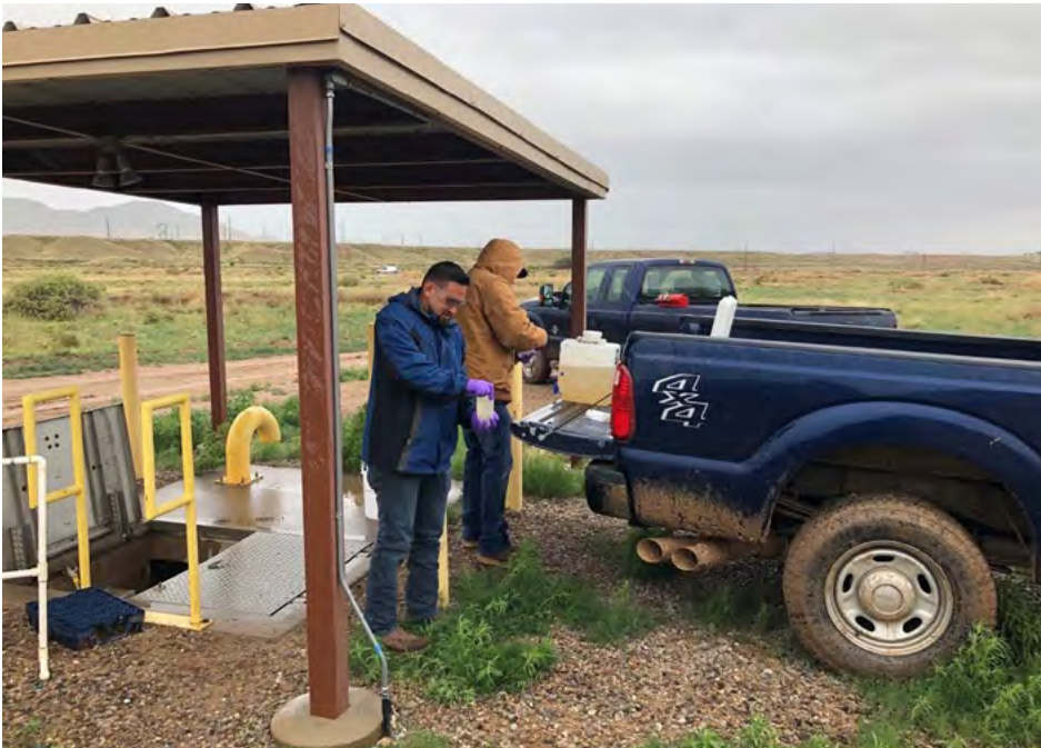
TESTING WASTEWATER — Environmental Field Team members collect samples of wastewater for laboratory analysis. The wastewater team conducts independent verification sampling to make sure Sandia meets water quality standards set by the Water Authority. Photo by Mark Zuverink
