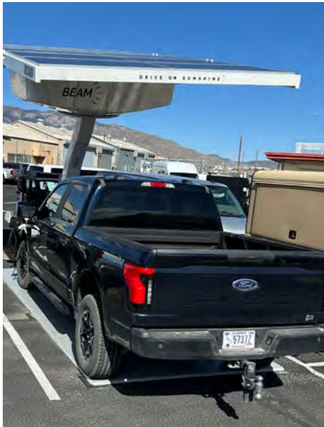
FEWER EMISSIONS — A Ford F150 Lightning “refuels” at an off-grid solar electric vehicle charging station.
