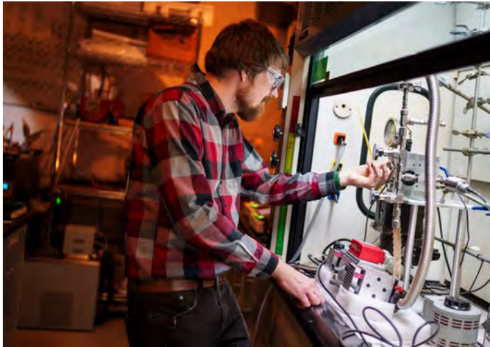
GASSING UP? — A geosciences engineer works on a gas adsorption system in a fume hood as part of a project to see if depleted petroleum reservoirs can be used for storing carbon-free hydrogen fuel.
