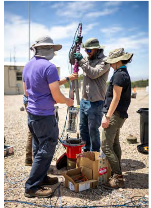
DOWN THE WELL — From left to right, electronics engineer Alfred Cochrane, electromechanical technologist Taylor Myers and mechanical engineer Melanie Schneider position a downhole acoustic transceiver and energy harvesting tool before lowering it into a well.
