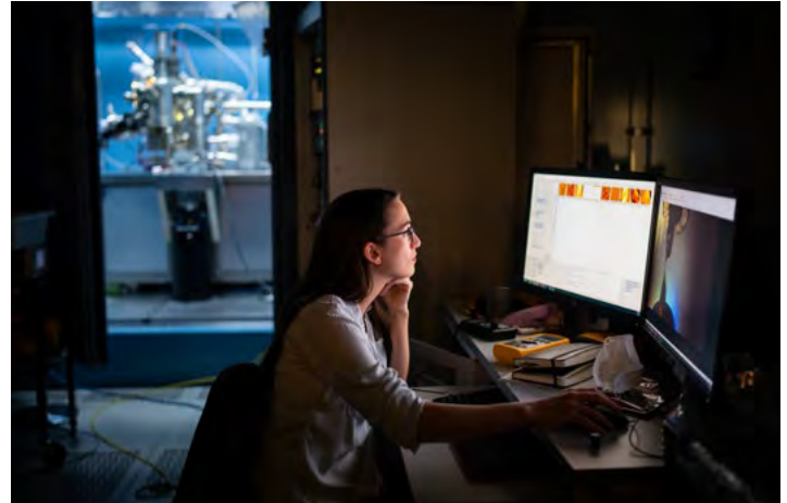
VANGUARD — Postdoctoral researcher Caitlin McCowan inspects pieces of silicon at the atomic level. She uses a scanning tunneling microscope to spot imperfections as part of a quantum research project at Sandia.
