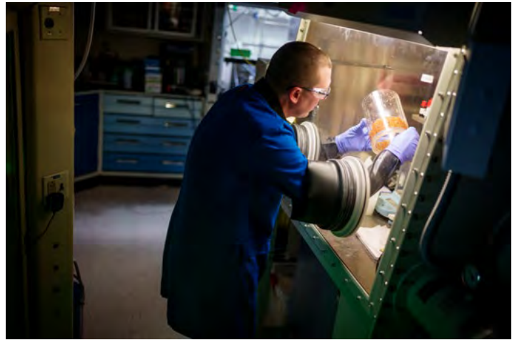
PREPPING PROTECTION — Sandia materials chemist Cody Corbin works in a glovebox, preparing a container filled with bead bits that will turn brown if someone attempts to tamper with the container’s contents.
