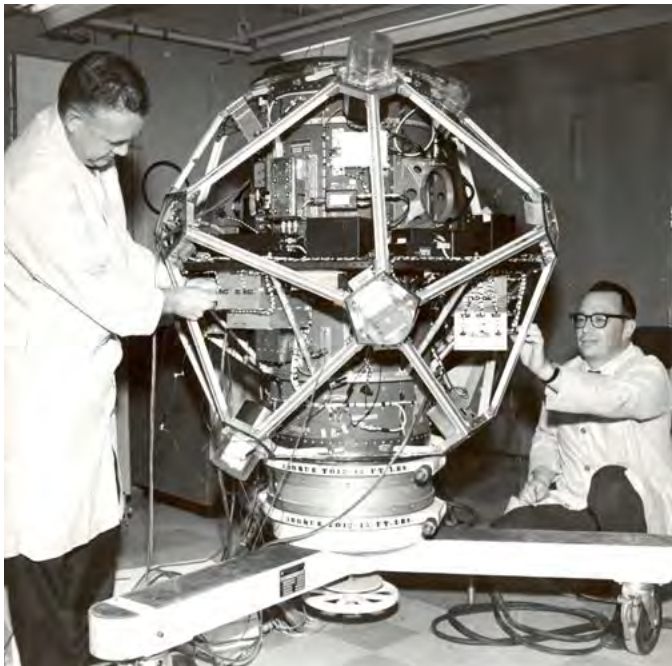
SATELLITE SHAKEDOWN — Bob House and Simon Steely putting the first Vela design through its prelaunch testing, 1963.
