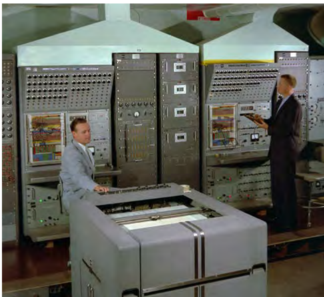
STATE OF THE ART — Sandia-designed, room-filling analog computer used for Vela simulation models. Archival Sandia photo
