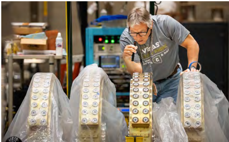
CHECK, CHECK — Each of the 20 high-voltage connectors on an inductive voltage-adder cell are being checked for assembly defects before moving the cell to electrical test.
