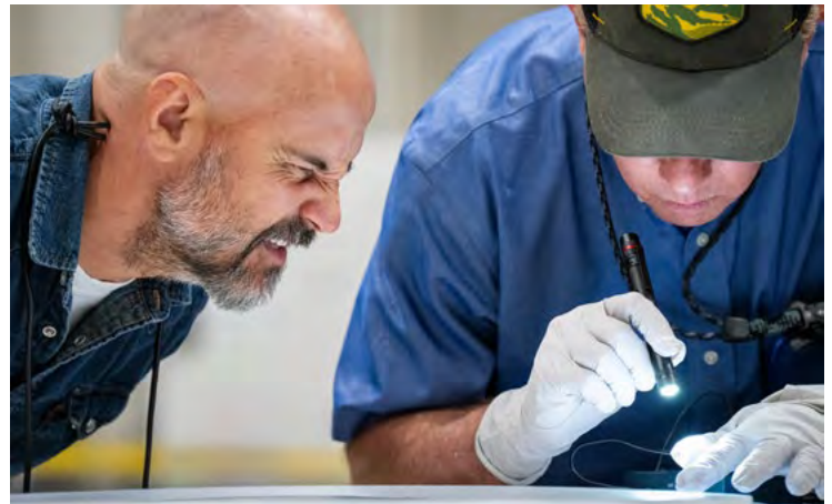
A CLOSE LOOK — An inductive voltage-adder insulator ring is being inspected for defects that could cause cell failure. After passing inspection, it will be assembled into a cell.
