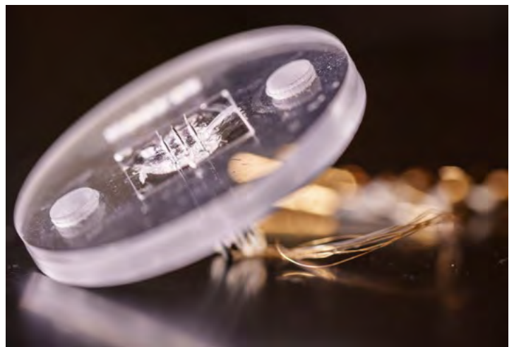
SMALL SENSOR SYSTEM — A microneedle-based sensor puck designed by Sandia researchers means quicker results for health care providers and less pain than a blood draw for patients. Photo by Craig Fritz
