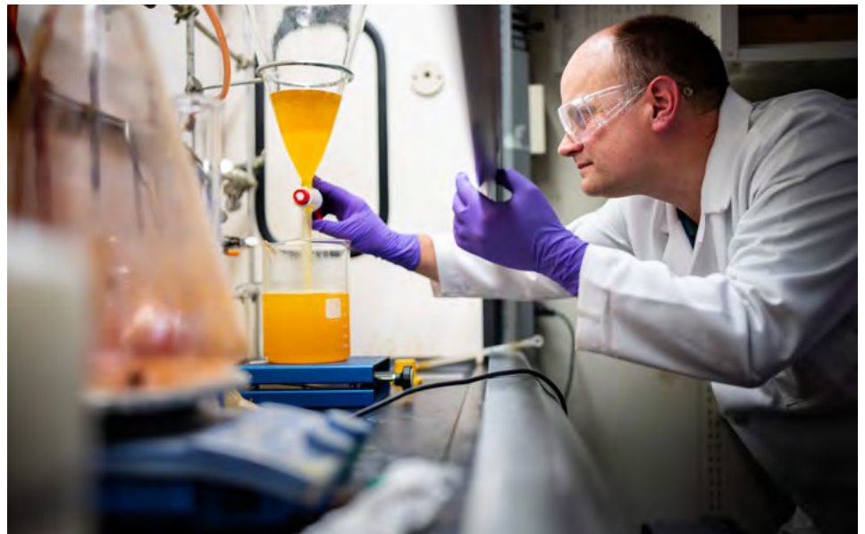
CHEMISTRY AT WORK — Sandia chemist Chad Staiger uses a separatory funnel to remove byproduct from the synthesis of a molecule. Photo by Craig Fritz
