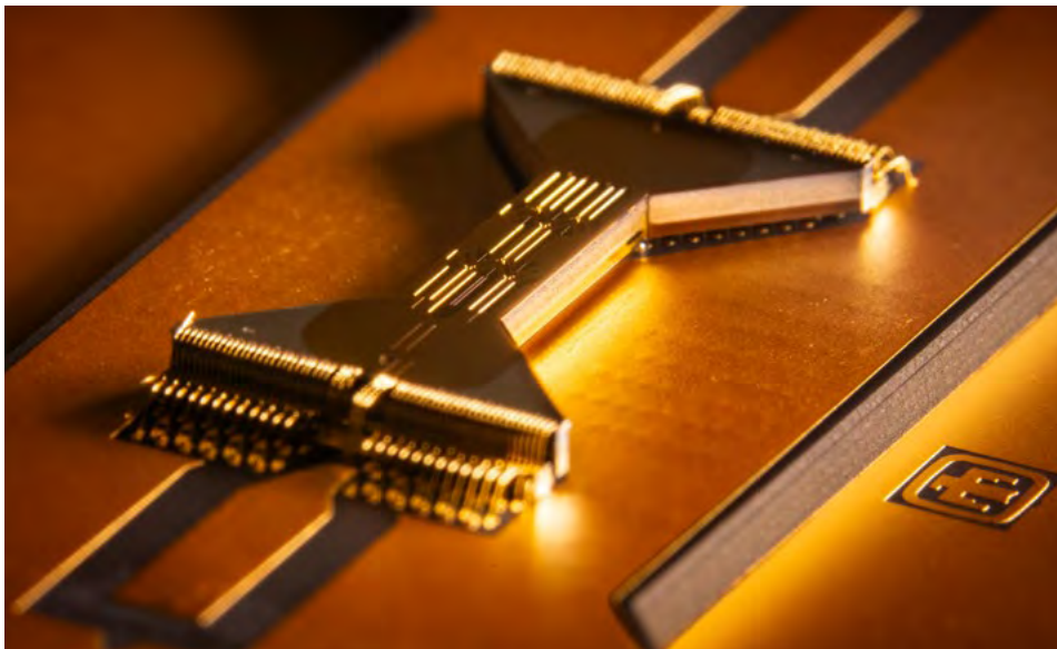
THE WHOLE ENCHILADA — The Enchilada Trap, manufactured in the Microsystems Engineering, Science and Applications fabrication facility. Photo by Craig Fritz
