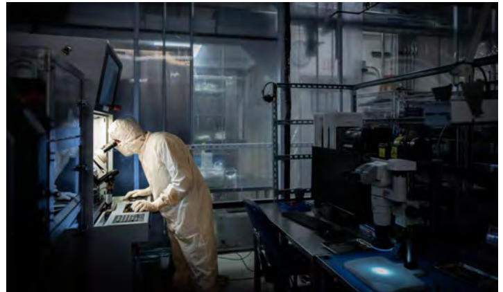
SETTING THE TRAP — Electrical engineer Ray Haltli optimizes parameters before placing gold wire bonds on an ion trap. When ready, the machine runs automatically, placing up to seven wires per second. Photo by Craig Fritz
