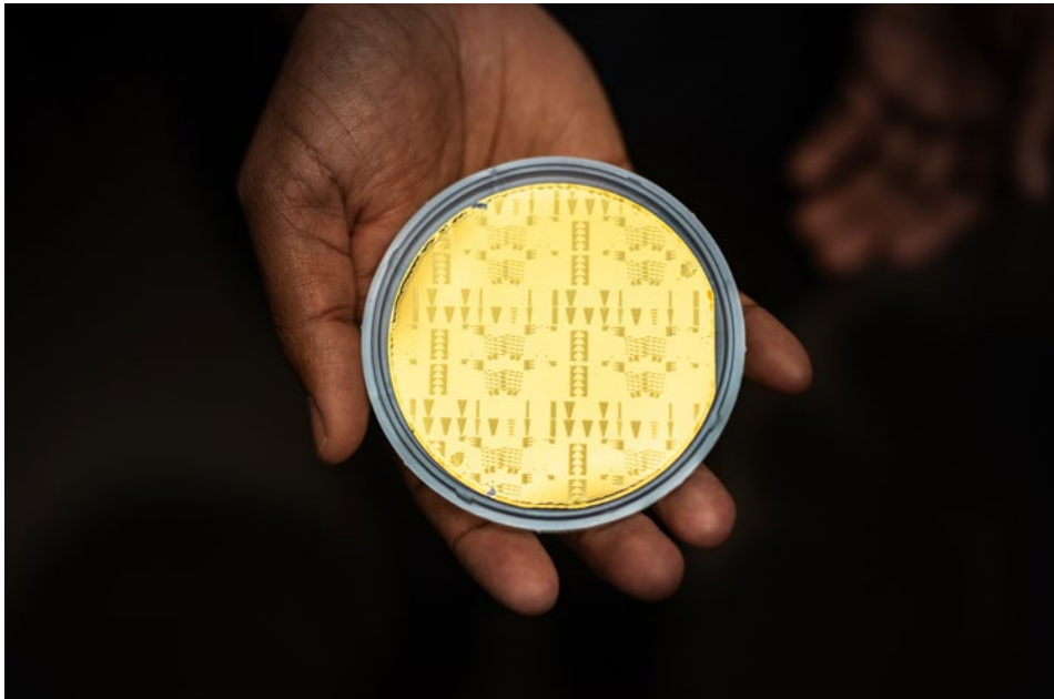
EXPERIMENTAL WAFER — More than a thousand experimental lasers and amplifiers adorn a three-inch, gold-electroplated silicon wafer made at Sandia's Microsystems Engineering, Science and Applications complex. Photo by Craig Fritz
