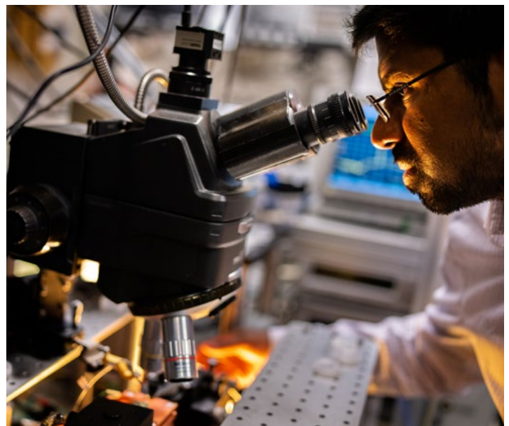
CHARACTERIZING LASERS — Sandia scientist Ashok Kodigala aligns a fiber to a chip-scale, heterogeneously integrated laser under a microscope at the MESA complex. Photo by Craig Fritz
