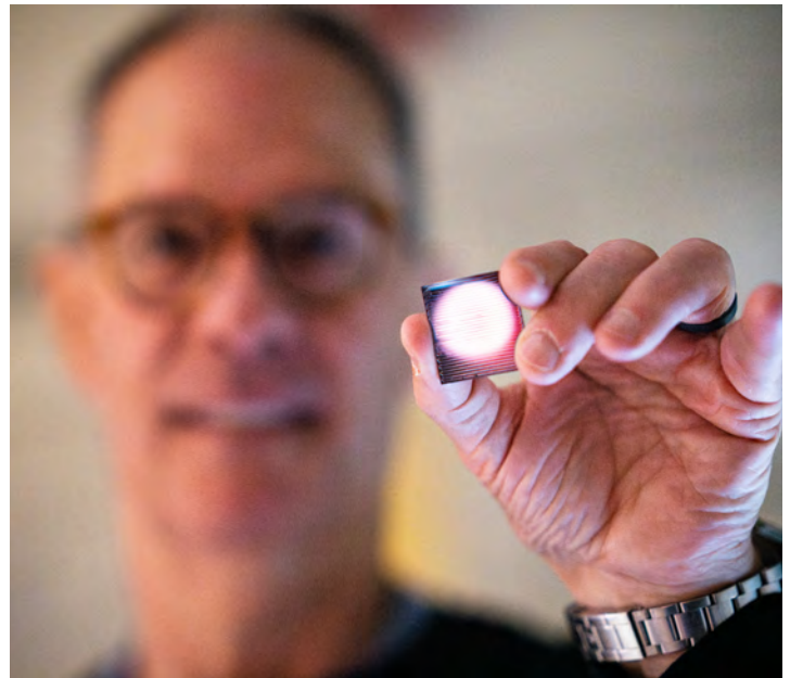
PUBLIC-PRIVATE PARTNERSHIP — Gary Arnold, CEO and founder of Know Biological, holds part of a miniaturized sensor system designed by Sandia biomedical engineers. The sensor can detect gases released from the skin of people with epilepsy before a seizure. Photo by Craig Fritz
