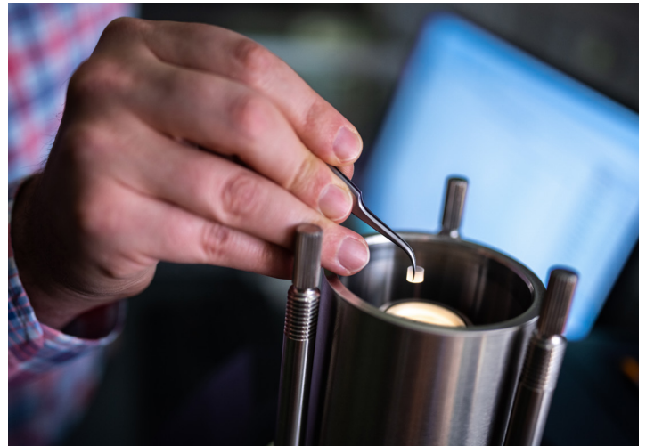
SAFETY FIRST — Chemical engineer Alex Bates places a sample into a differential scanning calorimeter. He’s part of a Sandia-led team working to predict the safety of advanced batteries while they are still under development.
