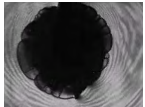
SHOCKING SCHLIEREN — A schlieren image of an experiment 80 microseconds after detonation. The image shows the leading edges, fingernail-like protrusions from the center, and emanating bands, lighter ripples. Sandia scientists hope this kind of data on fracture formation in plexiglass can be used to make geothermal energy more assessable. Image courtesy of Eric Robey
