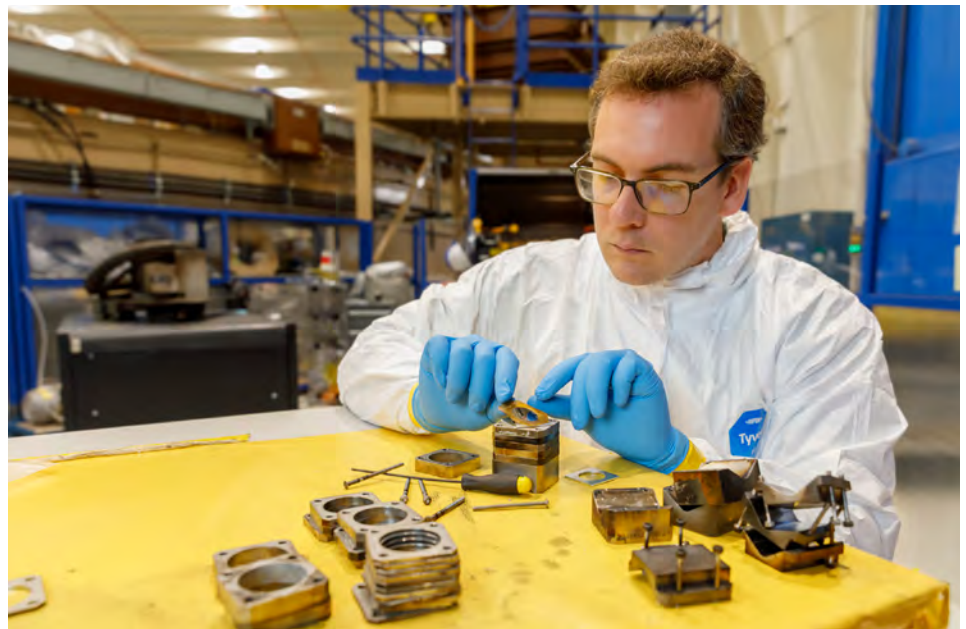
MATERIAL TEST — Physicist Chad McCoy at Sandia's Z machine loads sample coatings into holders. When Z fires, researchers will observe how well particular coatings protect objects stacked behind them.
