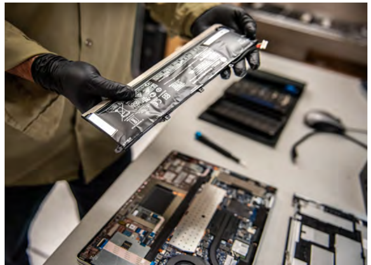
BULGED BATTERY — A swollen battery carefully removed from a Sandia laptop by the hardware repair depot team within IT Services.
