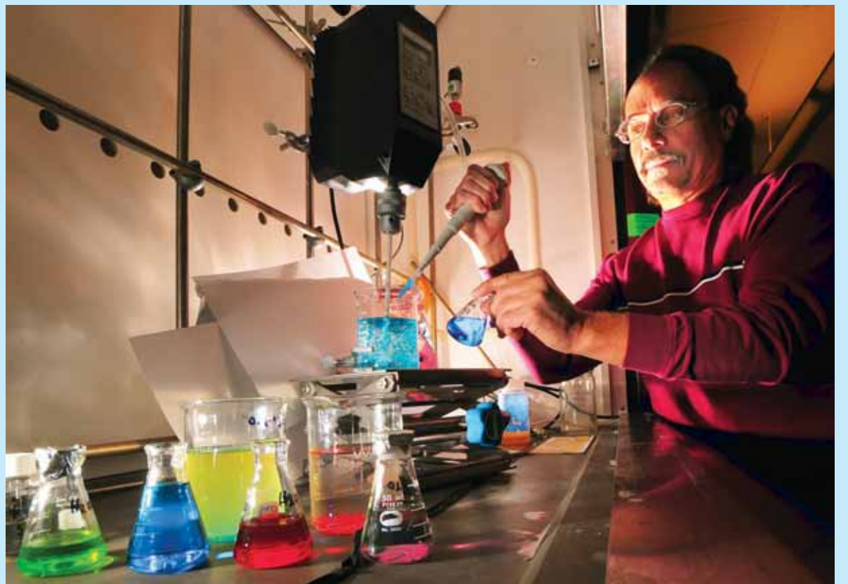
COLORFUL CALLING — Duane Schneider (2453) demonstrates a microencapsulation process that results in a chemical being encapsulated in a polymer shell. Familiar uses for microencapsulation include scratch-and-sniff perfume ads in magazines, time-release medications, and carbonless copy paper. Duane is working with a local business to develop a microencapsulation process for a cosmetics product. Read the story on page 5. (Photo by Randy Montoya)
