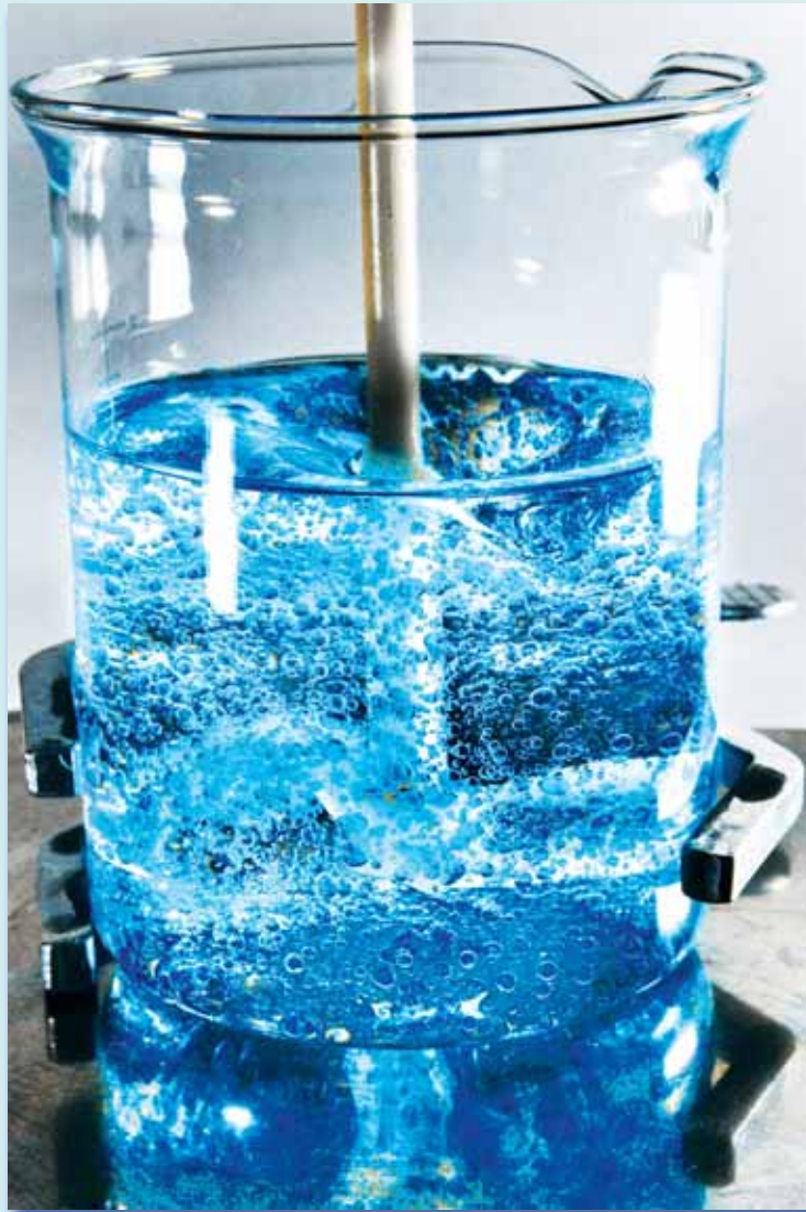
STIRRED, NOT SHAKEN — One frequently used microencapsulation process involves stirring an aqueous core and an organic solvent containing a dissolved polymer shell material into an emulsion. (Photo by Randy Montoya)
