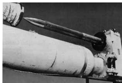
MARS PENETRATOR is tail-mounted upon air gun horizontally; breech of gun is fitted over it and the assembly raised to vertical position for firing.
