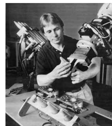
SHELL GAME — Walt Wapman adjusts a World War II-vintage anti-aircraft shell in a special tool assembly on a robotic arm.
