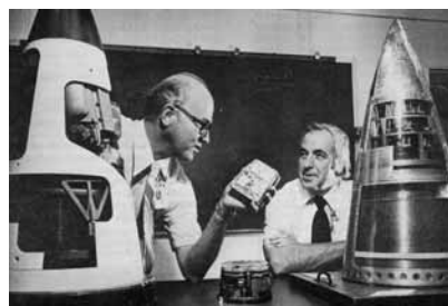
GETTING SMALLER, LIGHTER ALL THE TIME — Ray Alls holds Mk4 radar fuze as he talks to George Rodgers. Earlier radars were hefty items that occupied the middle third of these missile nosecones.
