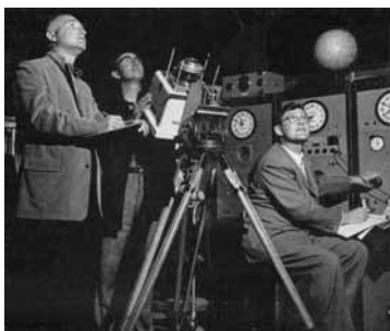
SATELLITE SEEKERS — Dan Parsons, left, takes notes while Dale Fastle prepares to photograph a satellite. Operating the radio console, which supplies accurate time information, is Ben Benjamin, who is in charge of the Sandia Phototrack Station.
