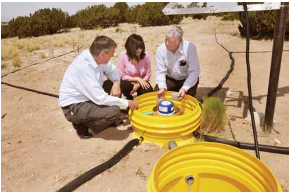
BOBBY CORBELL (5736), right, explains to representatives from NNSA's Sandia Site Office Sandia's approach to testing a Chaparral Infrasound sensor system at one of the FACT drill sites.
