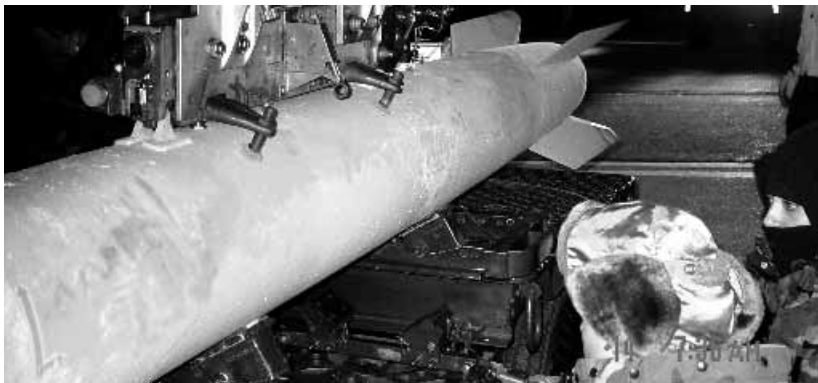
B61 FLIGHT TEST UNIT — a Joint Test Assembly — being preconditioned to cold temperature before flight at the Tonopah Test Range in Nevada.
