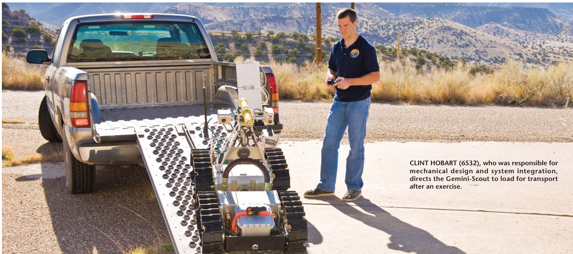
A-MAZING — Gemini-Scout can navigate through tight openings, up stairs and over rubble piles to reach trapped miners and assess any dangers rescuers might face.
