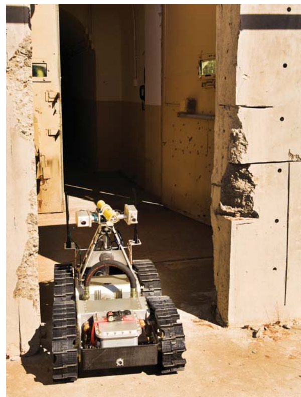
A-MAZING — Gemini-Scout can navigate through tight openings, up stairs and over rubble piles to reach trapped miners and assess any dangers rescuers might face.
