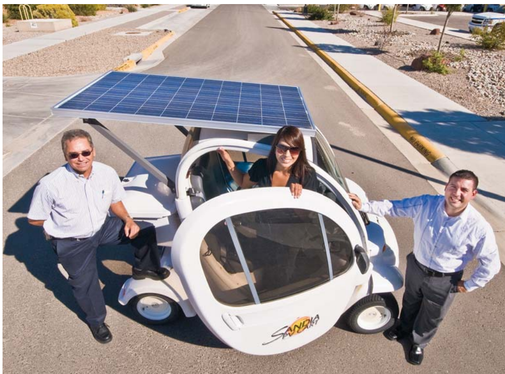
A SUNNY RIDE — Israel Martinez, left, Erika Barraza, and Matthew Brito (all 4821) were key members of a Sandia team that developed a photovoltaic-powered cart that won a 2010 Presidential GreenGov award. The cart is based on a modified GEM cart, familiar around Sandia's Tech Area 1. Members of the PV cart team were honored at a White House ceremony on Oct. 7. (Photo by Randy Montoya)
