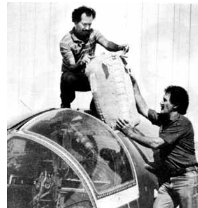
SANDIANS fit the chute cluster into an F-111 crew escape module.
