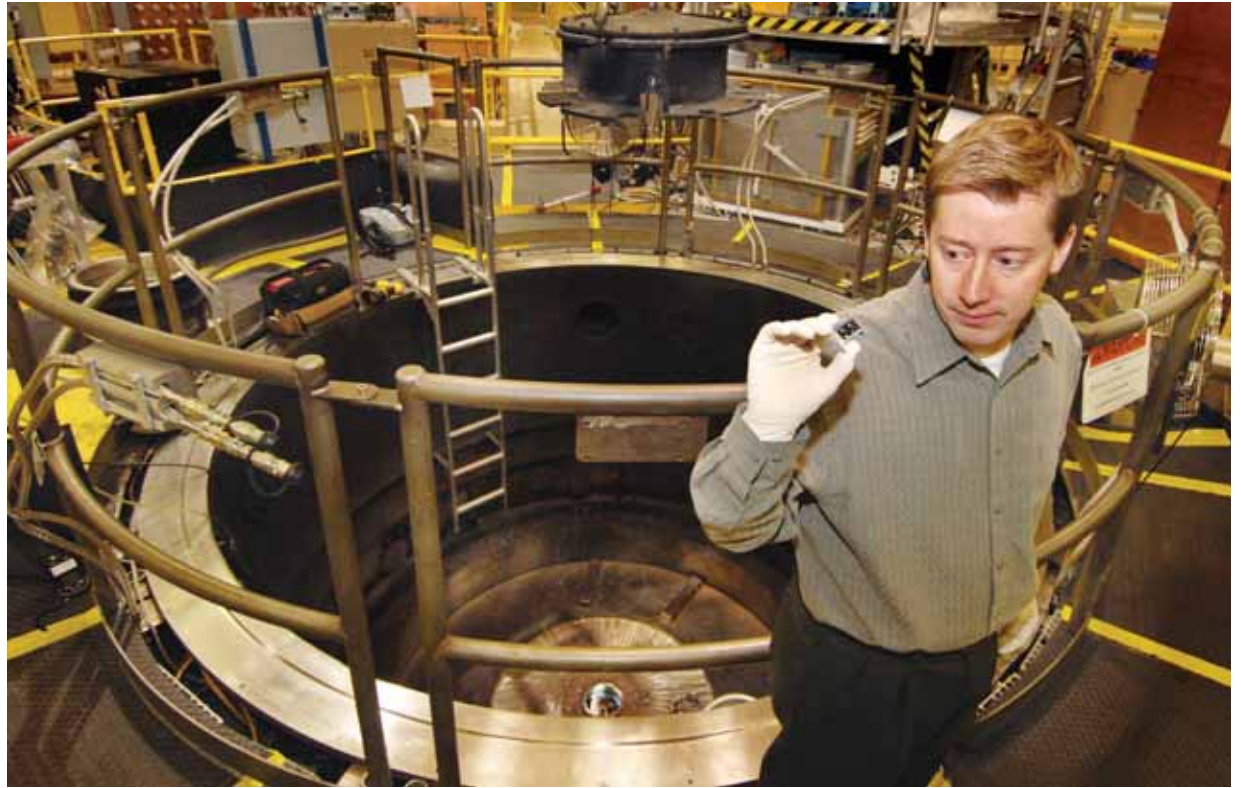
ARE YOU GOOD FOR ANOTHER 15 KM/SEC — Marcus Knudson considers his favorite apparatus — the Z insert that sends flyer plates hurling at phenomenal speeds. (Photo by Randy Montoya)
