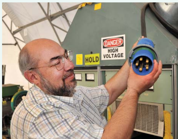
LEONARD MARTINEZ (1653) looks at the large twist-lock connector on an RF amplifier now at Reutilization and Disposition. Such machines have been used at Sandia since the 1970s in electromagnetic environment tests — this particular one at the Electromagnetic Environments Simulator (EMES). (Photo by Randy Montoya)
