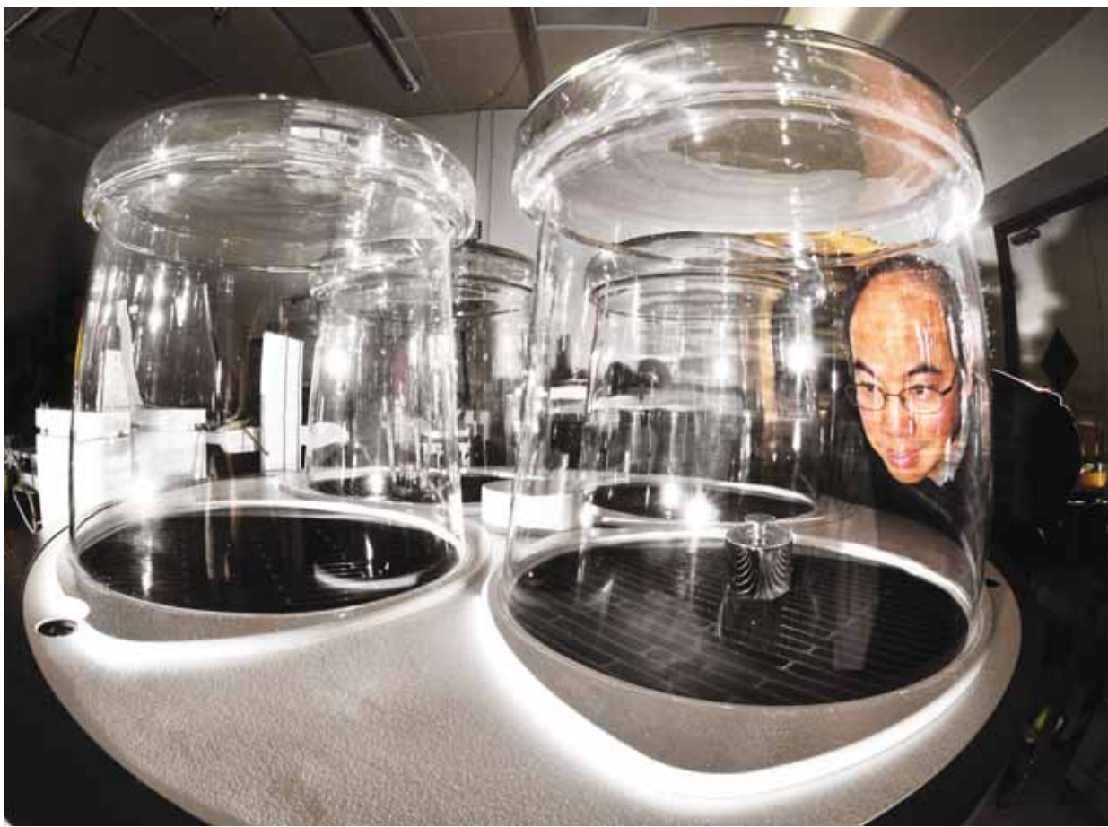
KILOGRAM UNDER GLASS — Mechanical engineer Hy Tran (2541) examines a kilogram sample in a mass comparator at Sandia's Primary Standards Laboratory. The international community is considering alternative means of defining the kilogram. (Photo by Randy Montoya)
