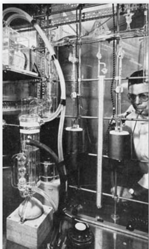
FINAL ASSEMBLY of an intricate glass vacuum system fabricated by Sandia's Glass Shop is made by Warren Roberts.
