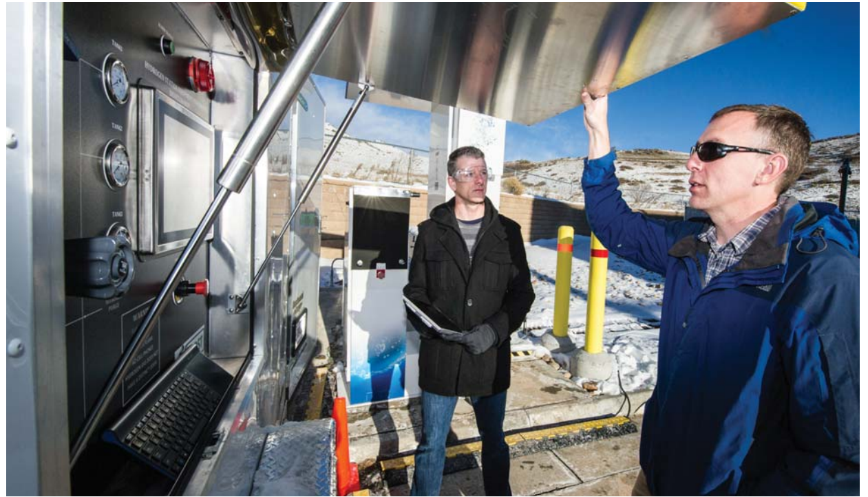
MECHANICAL ENGINEER Terry Johnson, left, the project leader for the Hydrogen Station Equipment Performance (HyStEP) device, and National Renewable Energy Laboratory researcher Chris Ainscough prepare HyStEP for testing at NREL's Energy Systems Integration Lab. HyStEP will accelerate hydrogen refueling station commissioning. (Photo by Dennis Schroeder/NREL)
