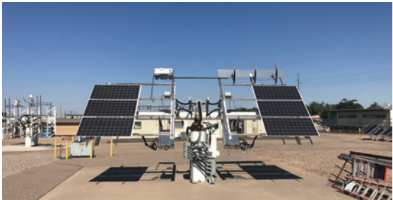
PHASE III — The final phase of the project involves side-by-side outdoor performance validation of Nishati’s prototype PV panels on Sandia’s unique two-axis tracking system.
