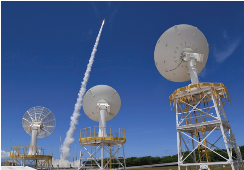
TAKING FLIGHT — A HOT SHOT sounding rocket takes off from Sandia’s Kauai Test Facility in Hawaii. Data collected from onboard sensors is allowing researchers to improve computer- and ground-based simulations of flight vibrations.
