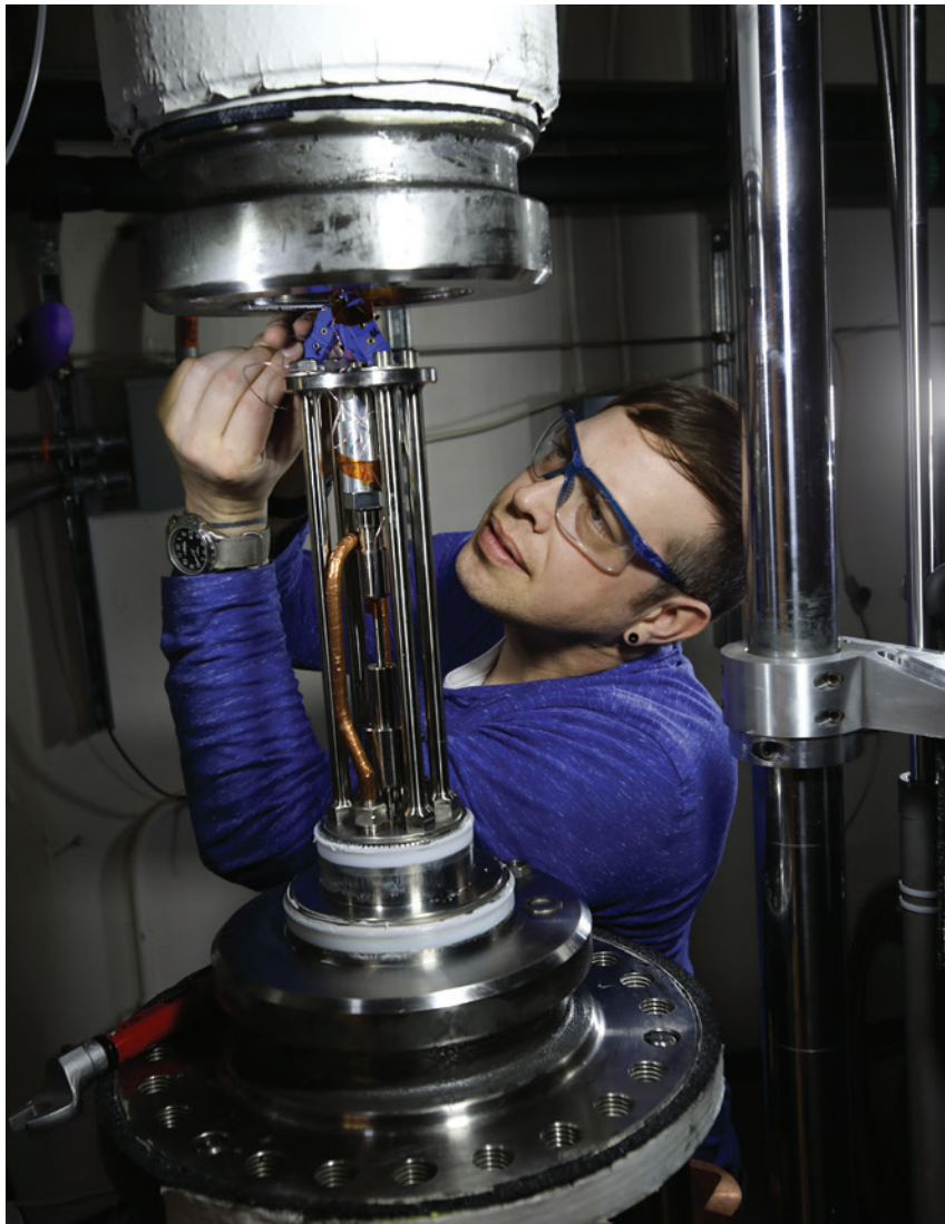
TESTING, TESTING — Principal high-pressure mechanical test systems designer and operator Brendan Davis prepares a system for testing hydrogen gas at Sandia’s hydrogen effects laboratory. Photo by Dino Vournas
