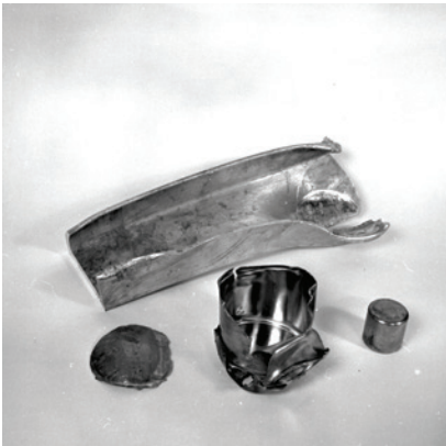
BEFORE AND AFTER — Sandia scientists tested a heat source with stainless steel outer container and aluminum mounting plate. The heat source was riveted onto the Apollo lunar surface instrument package.
