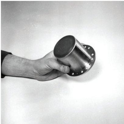
BEFORE AND AFTER — Sandia scientists tested a heat source with stainless steel outer container and aluminum mounting plate. The heat source was riveted onto the Apollo lunar surface instrument package.
