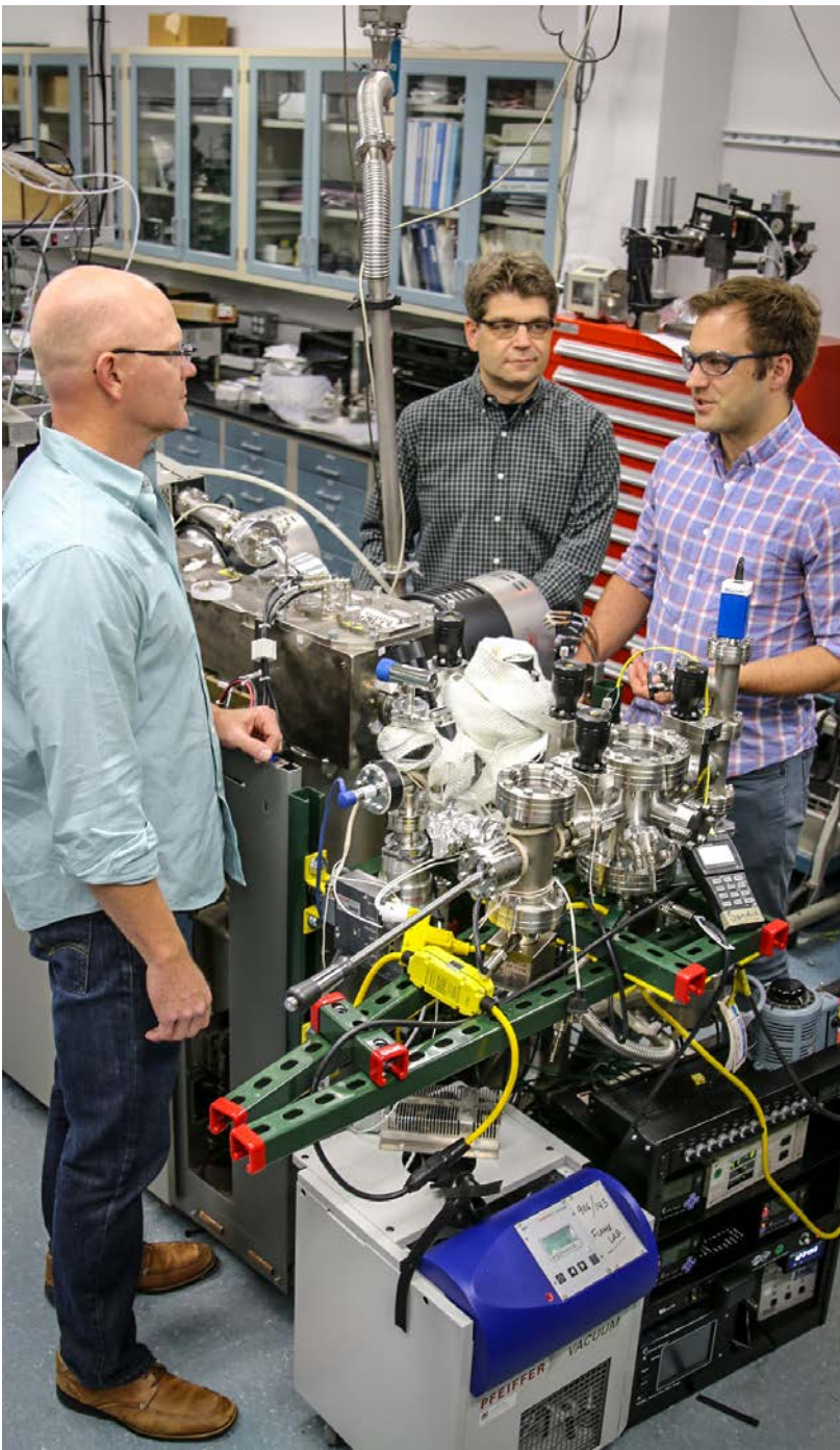
TALKING SOOT — Scott Skeen, Nils Hansen and Brian Adamson (left to right) discuss the tandem mass spectrometry technique they used to detect aliphatically linked polyaromatic hydrocarbons in a sooting flame.
